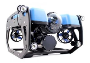
The BlueROV2 is a smooth, stable, and highly manoeuvrable mini ROV comprised of six thrusters, electronics and battery enclosures, and a rugged frame. Powerful but dimmable lights provide excellent illumination for the live HD video feed.
