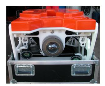
The ROV Pollux III is an observation class ROV fitted with an HD polyethylene frame and equipped with 4 electrical thrusters.
