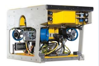
The Tomahawk is a 3000msw rated light work class ROV suitable for a large variety of tasks, including high speed survey & geophysics, Inspection Repair & Maintenance (IRM), drill and completion support / well intervention including fluid injection, AX/VX and torque tool capability, light intervention & construction, pre/post pipe & cable lay survey, touch-down monitoring and diver support tasks plus many other oil & gas, renewable energy, civil engineering, military or scientific mission.
